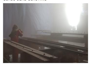
VIVABLAST is one of the few providers of glass bead blasting in the industry, which does not cause so much erosion on the surface of a coater while it is being cleaned. We were asked to provide the manpower, also material and specialised equipment to successfully do the cleaning of a full set of coaters for one of our valued manufacturing client. We ensured these were resized and fully cleaned to provide continued efficiency.
